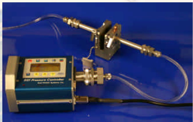
Controlling Pressure on 1/2" Weld
