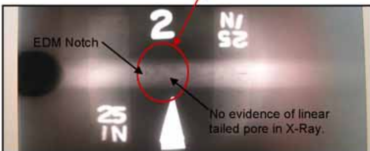
X-ray of Fuel Line Weld
