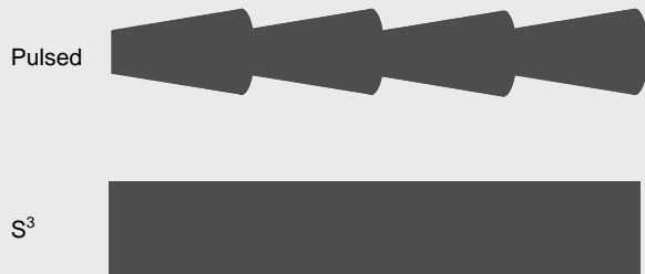
Image 3, Pulsed Weld Christmas Tree Effect vs. S 3
